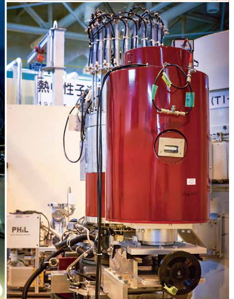
(Left) An overall picture of POLANO spectrometer which can measure the spin and lattice dynamics with polarized neutron beam. (Right) Advanced KINKEN Triple-Axis Neutron Spectrometer (AKANE).
